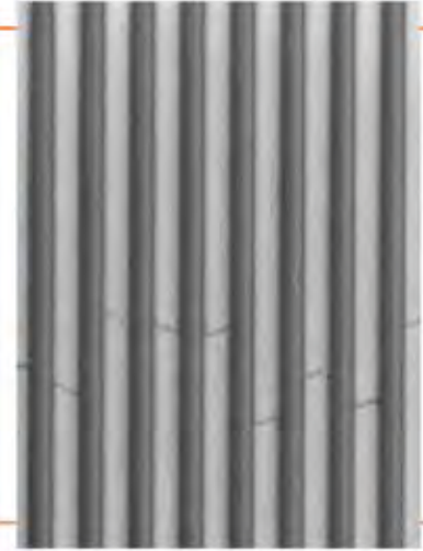
SEM Image of riblets created by laser in a commercial aerospace paint system
